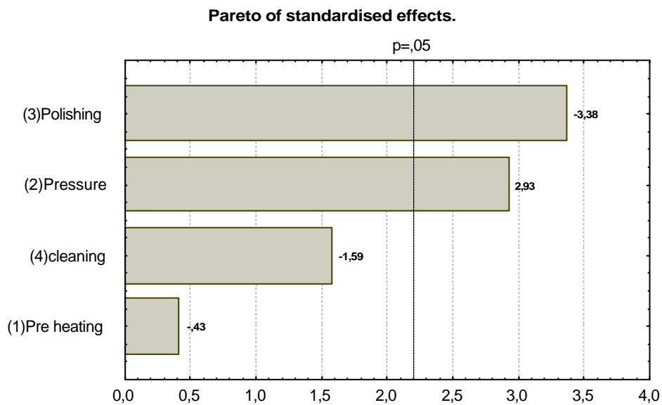
Figure 6: Effect of factors on strength of connection. The negative value for polishing shows that polishing results in lower strength. The same goes for wet cleaning (less significant). Increased tool pressure has a positive effect.
